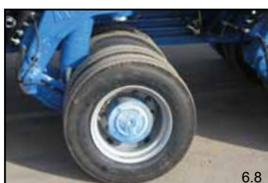
Hydrostatic wheel drive in the twin-tyred pendulum axles
