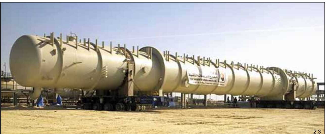
Transport of a 110 tons and 56 m long column 2.3
