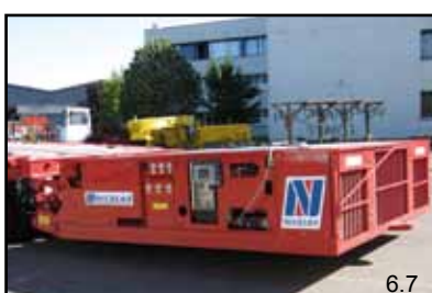
PowerPackUnit provides power for drive, lift and steering
