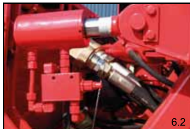
Centering actuator for raising and lowering the PowerPack-Unit
