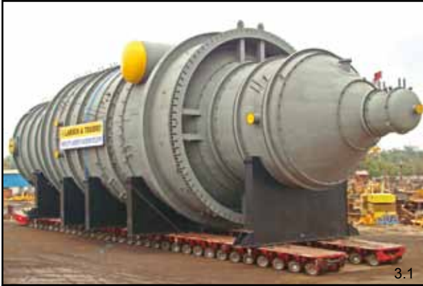
3.1 Transport of the world's largest vacuum column
