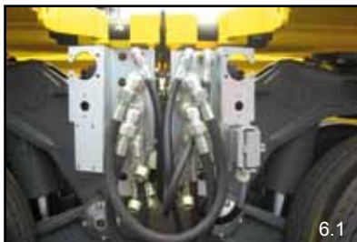
Connection of hydraulics and electronics through quick-release couplers
